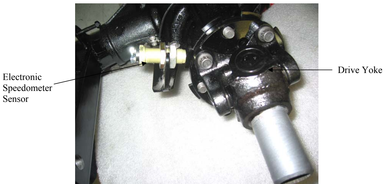
Drive yoke and Electronic Speedometer Sensor Fig. 8-5
