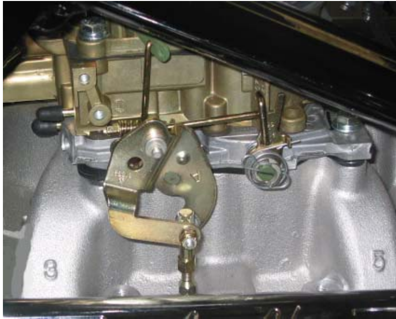
Throttle Linkage Connection at Carburetor Fig. 5-3
